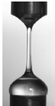
Figure 2-1: Liquid filament bridge is formed between two plates after application of a step strain.
