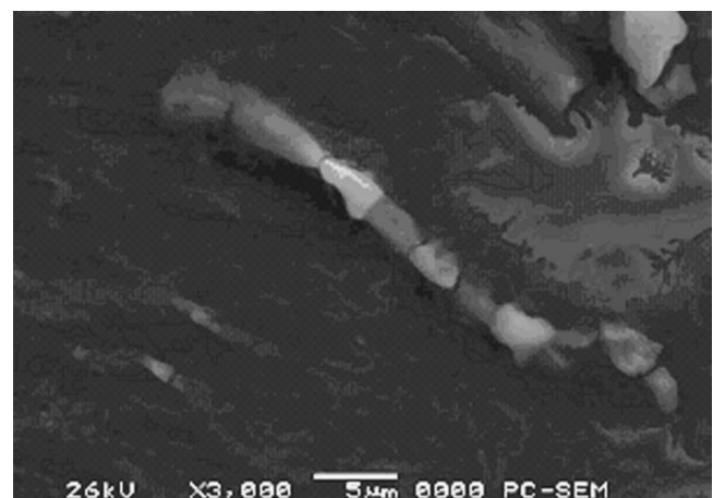
Fig. 3 SEM of bamboo structured ferrofluid nanoparticle–CNT composite
