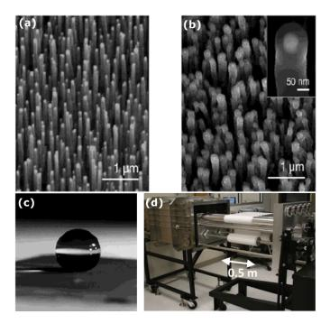
**Fig 11.** SEM images of (a) as as-grown carbon nanotube forest, (b) a carbon nanotube forest conformally coated by a 50 nm thick PTFE layer deposited by iCVD, and (c) a spherical water droplet on the PTFE-coated carbon nanotube forest. (d) Schematic of a roll-to-roll iCVD system for the hydrophobization of large scale substrates. Figures are reproduced from the hydrophobization of large scale substrates.
