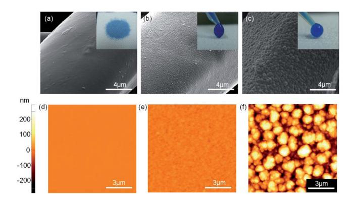
**Fig 12.** SEM and AFM images of (a & d) a non-coated polyester fabric surface, (b & e) a slightly rough PV4D4/PPFDA) stacked polymers iCVD-coated fabric surface and (c & f) a rougher surface of the PV4D4/PPFDA stacked polymer iCVD-coated fabric surface. Inset images show water droplets on the respective surfaces. <sup>174</sup> Figures are reproduced from <sup>174</sup> with permission from RSC.
