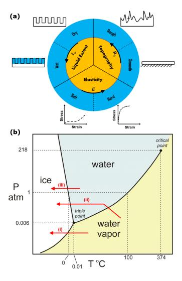
**Fig 1.** (a) A framework for classifying recently developed icephobic coatings. (b) Phase diagram for water indicating three different pathways for formation of water-based solid by changes in temperature and/or pressure of water. (i) vapor-solid or deposition, (ii) vapor-liquid-solid or condensation followed by freezing, and (iii) liquid-solid or freezing.
