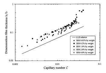
FIG. 9. Dimensionless film thickness versus capillary number for various bulk concentrations of SDS.
