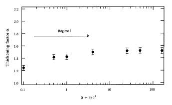
FIG. 6. Thickening factor  $\alpha$  vs  $\phi = c/c^*$  for BSA solutions. The concentration  $c^*$  is where multilayer formation begins.
