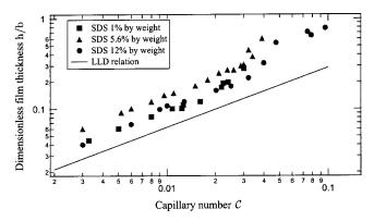
FIG. 11. Dimensionless film thickness versus capillary number for SDS at very high concentrations.
