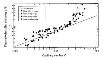
FIG. 14. Dimensionless film thickness versus capillary number for Elmer glue solutions.
