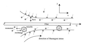
FIG. 1. Sketch of a fiber passing through a fluid bath. The presence of surfactants at the interface and in bulk as monomers and micelles is also indicated.
