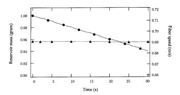
FIG. 3. Experimental data of reservoir mass (left ordinate) and fiber speed (right ordinate) versus time. Every fourth data point is indicated by a symbol. SDS solution (0.2% by weight) with fiber speed 0.69 m/s.
