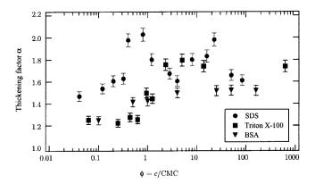
FIG. 12. Thickening factor  $\alpha$  for three surfactants BSA, Triton X-100, and SDS. For BSA interpret the CMC as the concentration at which multilayers form.
