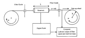
FIG. 2. Sketch of the experimental setup. The film thickness is determined by monitoring the mass loss from the fluid-filled reservoir.
