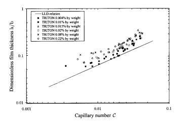
FIG. 7. Dimensionless film thickness versus capillary number for various bulk concentrations of Triton X-100.
