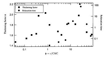
FIG. 13. The thickening factor (squares) for SDS plotted as a function of concentration and overlayed with the data for micelle lifetime (circles) for SDS obtained by Patist *et al.* (Ref. 21).
