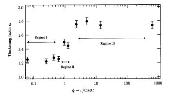
FIG. 8. Thickening factor  $\alpha$  vs  $\phi = c/\text{CMC}$  for Triton X-100 solutions.
