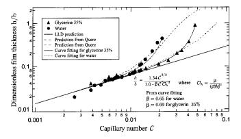
FIG. 4. Film thickness versus capillary number for a solution of 35% glycerin by weight in a water solution and for pure water. The solid lines are the best fit using Eq. (5). The dotted lines are obtained using Eq. (6).
