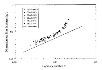
FIG. 5. Dimensionless film thickness versus capillary number for various bulk concentrations of BSA.
