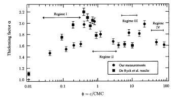
FIG. 10. Thickening factor  $\alpha$  vs  $\phi = c/\text{CMC}$  for SDS solutions.
