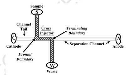
Fig. 1. A schematic of a conventional microdevice illustrates an 11-cm-long separation channel, a "double-T" cross-injector configuration, and channel tail section. The sample channel is depicted on the upper left-hand side of the image while the waste channel is shown on the lower right-hand side. Cathode and anode reservoirs are denoted by "C" and "A", respectively, as are the sample, "S", and waste, "W", reservoirs. The frontal and terminating boundaries of the DNA sample are also identified.
