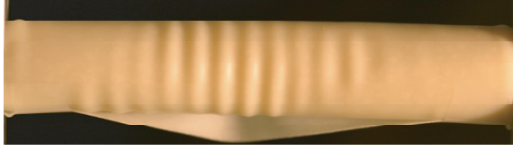
Fig. 3 – When the voluted rubber scroll is compressed axially, a rippling pattern similar to the one in Fig. 1 appears. A calculation similar to the one in the text then leads to the following expressions \lambda = 2\pi(tR)^{1/2}/\sqrt{3} \approx 3.6(tR)^{1/2} , A = \lambda(\kappa R)^{1/2}/\pi^{1/2} \approx 1.46R(t\kappa)^{1/2} , and yields results in agreement with observations. The small difference in the amplitude from the result for the bent tubes arises from the difference in the strain distribution in the two cases; however the wavelength remains the same. We note that this configuration is energetically unstable for isolated thin cylindrical shells which prefer to buckle into an almost inextensible surface patterned by diamond-like buckles; here however, the multi-layered structure stabilizes the axisymmetric state.
