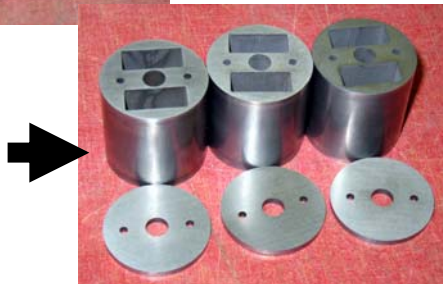
Tungsten Holders for Bend-Bar and Tensile Specimens
