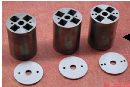
Tungsten Holders Thermal Diffusivity Specimens
