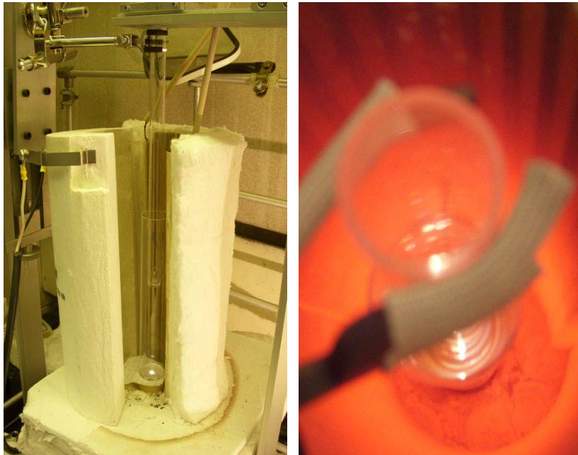
Salt Variable Optical Path Length Transmission Apparatus (850°C)
