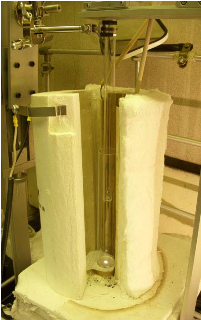
Salt Variable Optical Path Length Transmission Apparatus (850°C)
