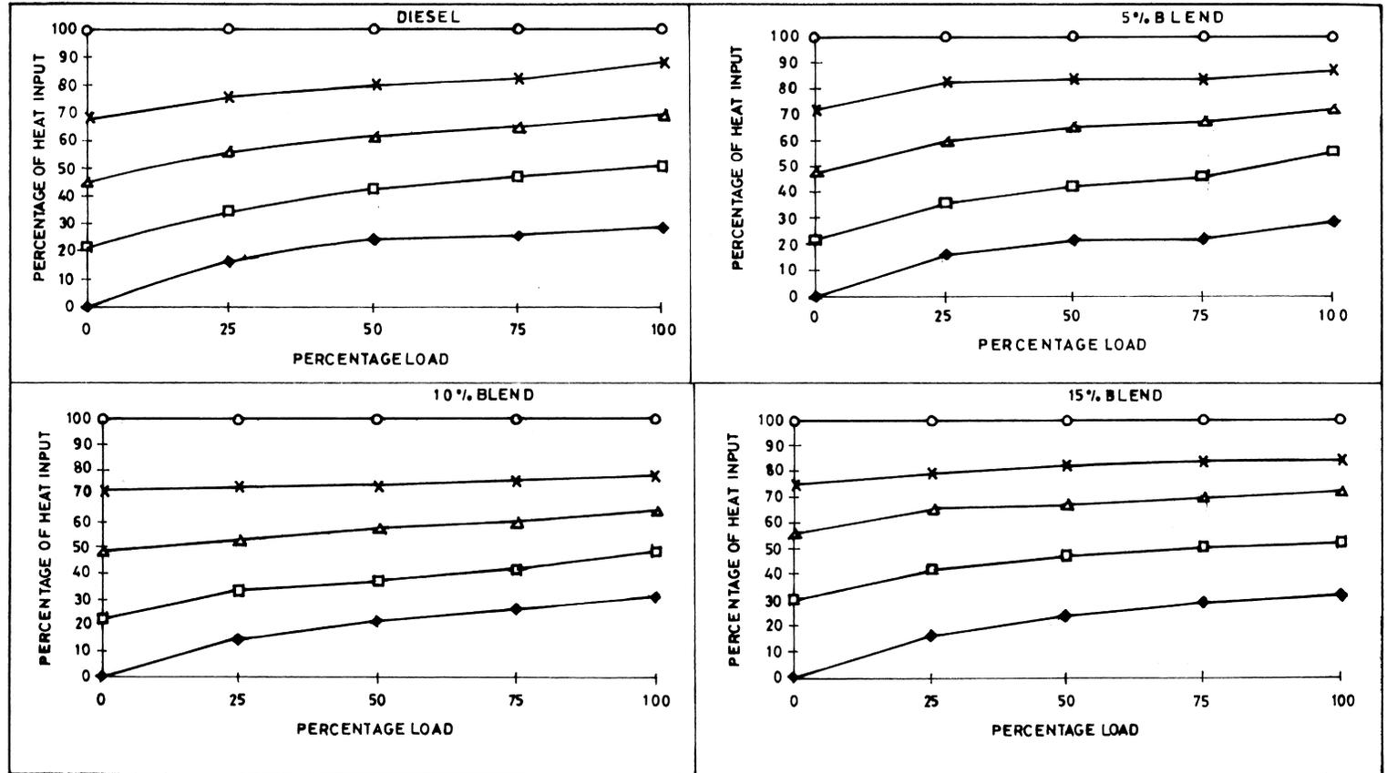
Fig. 2. Thermal balance of engine operating on diesel, 5, 10 and 15% ethanol-diesel blend.
