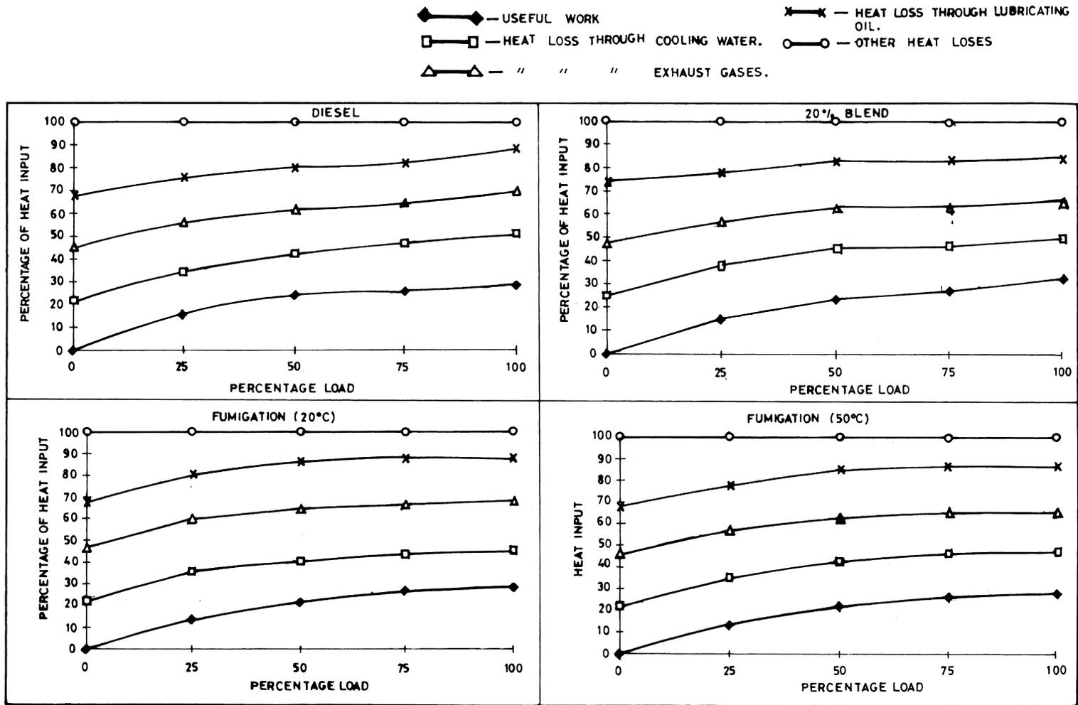
Fig. 3. Thermal balance of engine operating on diesel, 20% blend and fumigation.
