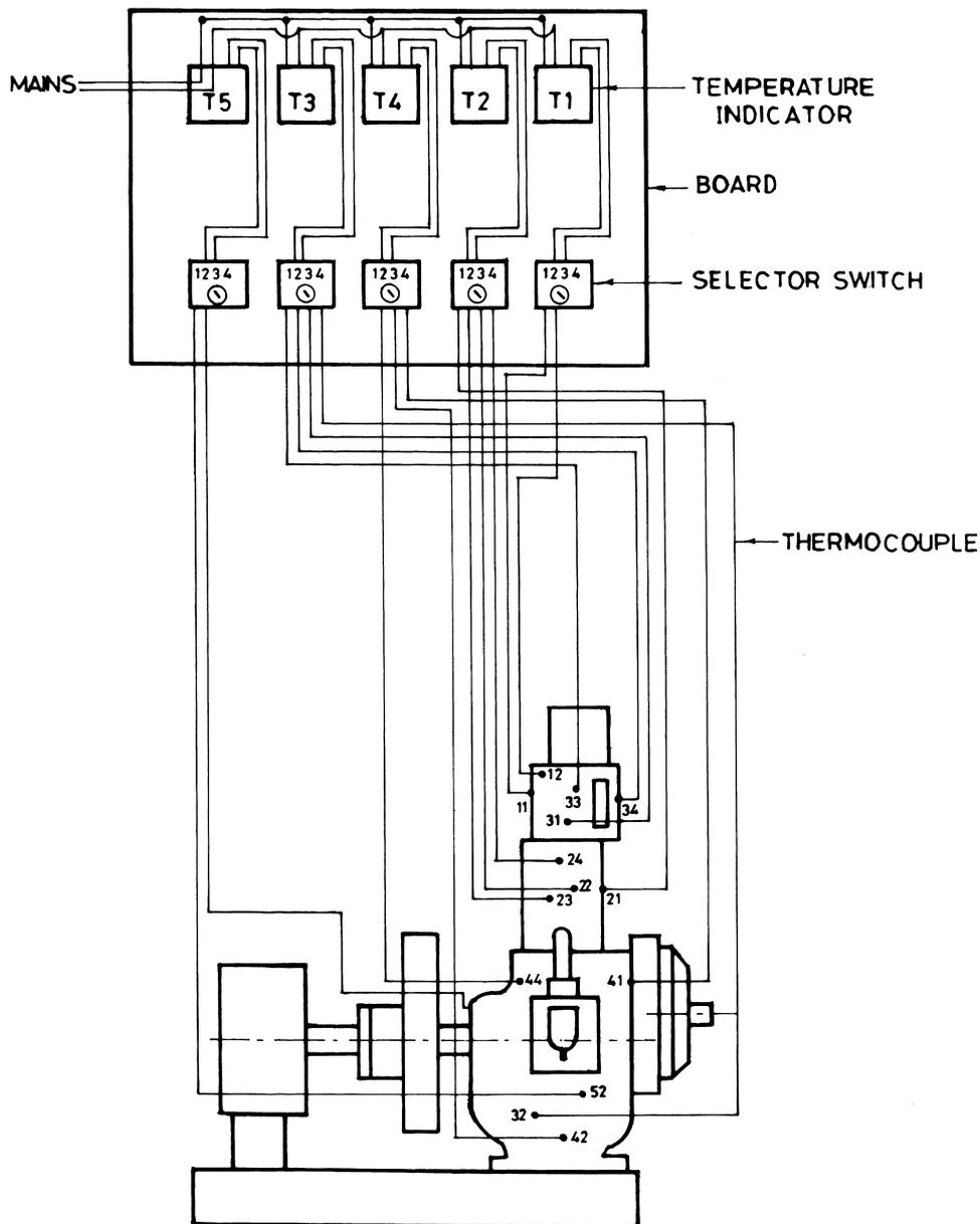
Fig. 1. Thermocouple connections for temperature measurements at various points of the engine.
