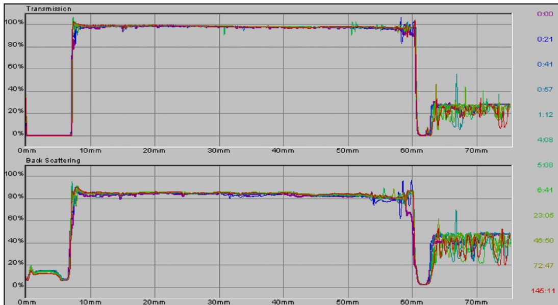
Fig. 1. Transmission (above) and backscattering (below) profiles for a stable sample.
