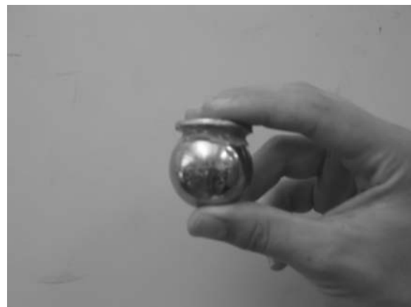
Figure 5 Vehicle Dropper Markers. These markers have proven to be robust and reliable.
