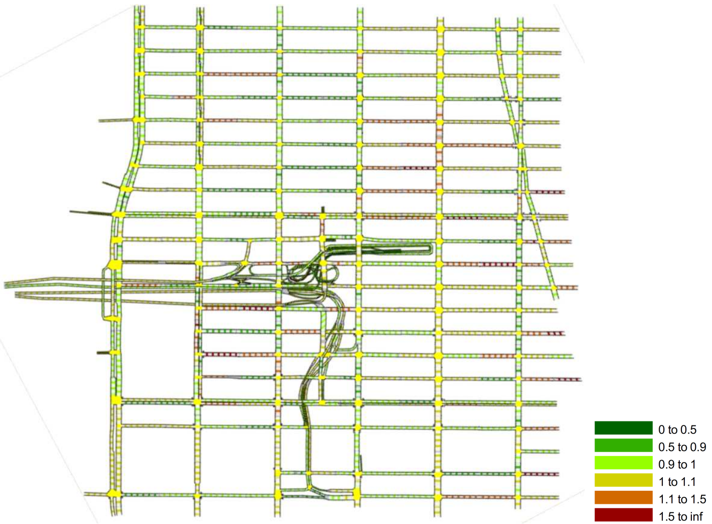
Figure 8: Ratio of the average link density under the proposed plan and that under the existing plan
