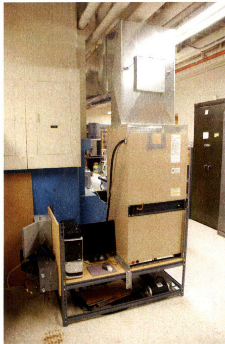
Figure 2-22: Picture of the overall air handler apparatus and attached duct system.
