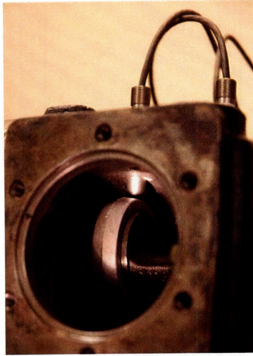
Figure 3-25: Closeup picture of position sensors.
