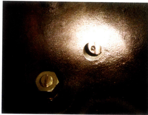
Figure 3-27: Set screw and connecting rod viewed from outside the crankcase through the position sensor mounting hole with position sensor absent.
