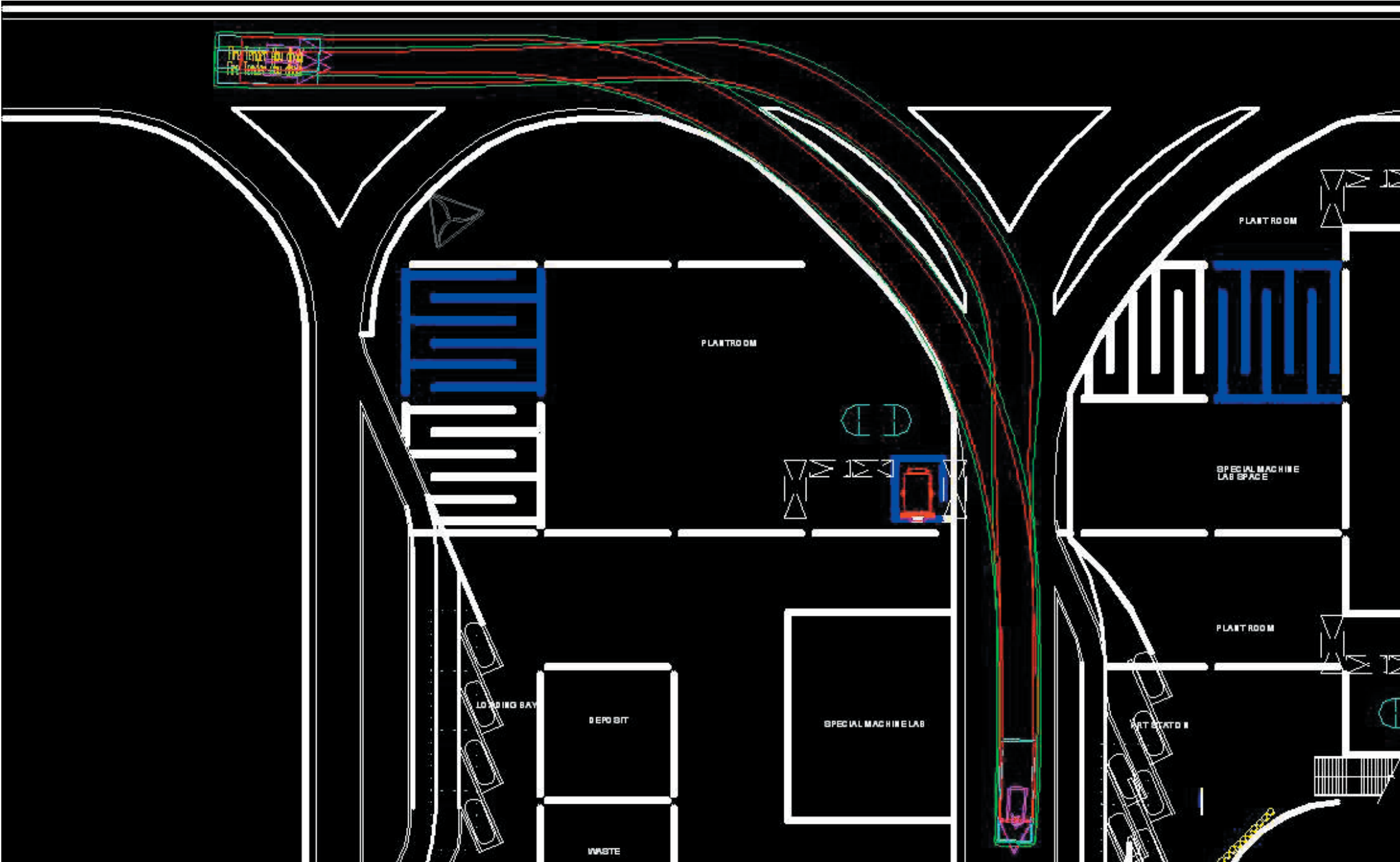
AD fire truck swept path verification in the undercroft structure (35km/h)
