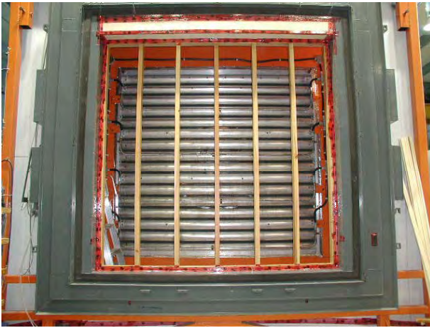
Figure 10- Installation of the wood-stud frame in EEEF
