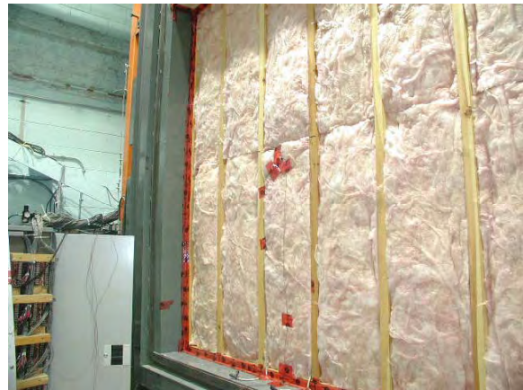
Figure 15 - Installation of insulation in stud-cavity
