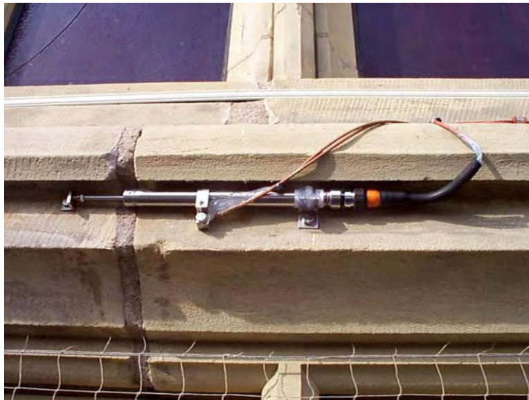
Figure 3. A photo (PT991119) showing a displacement sensor tucked under a windowsill to monitor movement across a repaired crack.
