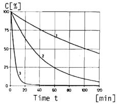
The effect of window aperture on the air change in a residential unit (test building D in Table I) under uniform wind conditions (north wind v about 3-4 m/s) and for an indoor/outdoor temperature difference of 15 K.
