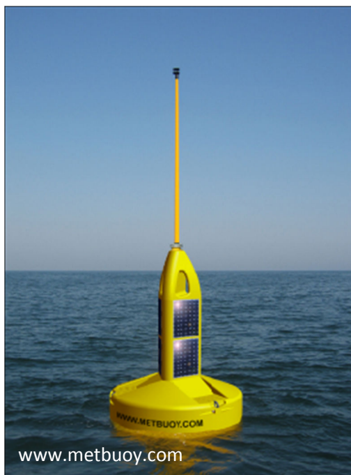
Figure 2-1: A photo of a typical buoy used for meteorological data collection from a company called Marine Data Service
