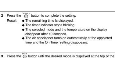
You can set the On Timer to turn on the air conditioner automatically at the appointed time. You can set the time from 1 hour to 24 hours.
