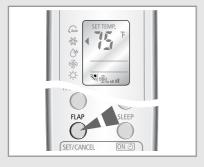
You can adjust the airflow direction vertically. The outer airflow blade moves up and down to increase the efficiency of the cooling or heating operation.
