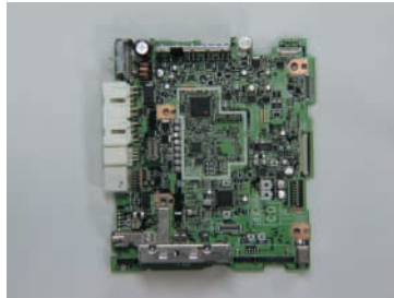
Main circuit board that uses lead-free solder
