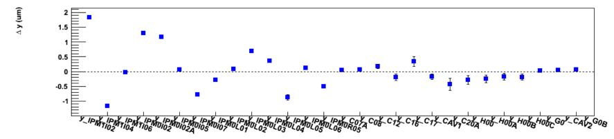
Turn ON position feedback: Zero position differences in Injector at 0L05 and 0L06
