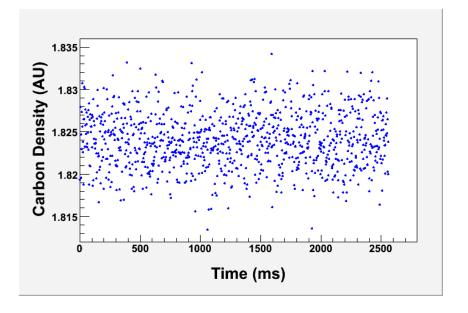
✓ Cryogenic target boils when heated by electron beam. For QWeak: 180 µA on 35 cm liquid hydrogen target (2.5 kW heat load)
