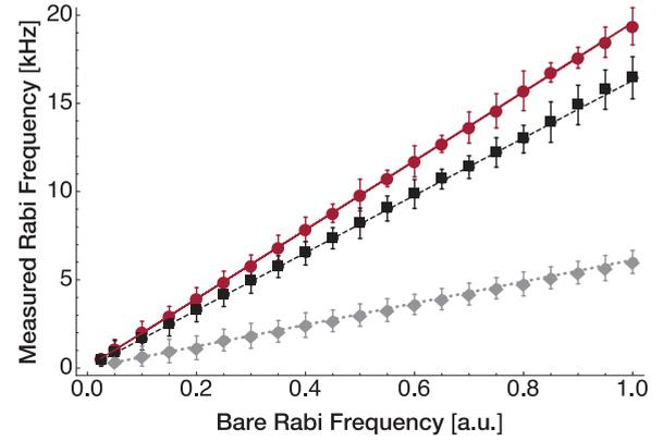
FIG. 4. (Color online) Measured enhanced  $^{14}\text{N}$  Rabi frequency in the three NV manifolds (red solid line,  $m_s = 0$ ; black dashed line,  $m_s = -1$ ; gray dotted line  $m_s = +1$ ) as a function of the bare Rabi frequency at  $B = 509$  G.
