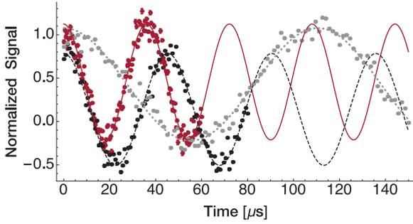
FIG. 2. (Color online)  $^{14}\text{N}$  Rabi oscillations at  $B = 450$  G,  $B_1 \approx 3.3$  G in the three NV manifolds (red solid line,  $m_s = 0$ ; black dashed line,  $m_s = -1$ ; gray dotted line,  $m_s = +1$ ). Here, the dots are the experimental results, while the lines are fits to cosine oscillations. The different baseline of the  $m_s = -1$  curve is due to small differences in the fluorescence emission of different nuclear manifolds [36].
