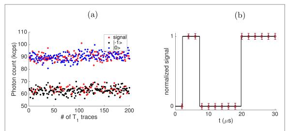
**Figure A2.** Engineered  $T_1^e$  measurement. (a) We compare the measured NV fluorescence at a fixed time,  $t=16~\mu s$ , to the 'bright' and 'dark' reference lines, given by the population states  $|0\rangle$ ,  $|-1\rangle$ , for all 200 different traces. We clearly see that the final state can be read out with high fidelity. (b) One of the engineered  $T_1^e$  trace of theory (black solid line) and experiment (red diamond). Error bars are one SEM.
