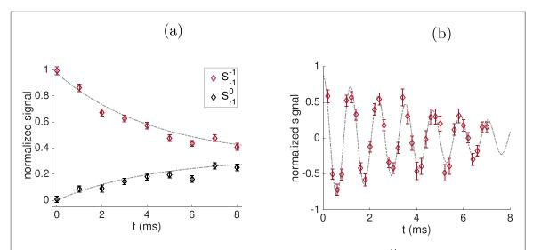
**Figure 2.** (a) Natural relaxation decay of a single NV population and (b) coherence decay of its native <sup>14</sup>N under a Ramsey sequence. The dashed lines are fits to the expected dynamics, yielding  $T_1^e = 4.3(3)$  ms and  $T_2^{*n} = 5.6(1.7)$  ms. These values satisfy  $T_2^{*n} = 1.5T_1^e$ , as predicted by the spin fluctuator model. All error bars in the figure are one standard error of the mean (SEM).
