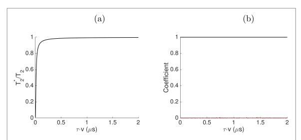
Figure B3. Contribution of different eigenvalues in the  $T_2^n$  decay with a 3-level RTN, for weak fluctuator. (a). Decay rate corresponding to the slowest decaying eigenvalue as a function of the DD interval  $\tau$ . (b) Contribution of each eigenvalue to the qubit coherence. We see that only the black line corresponding to slowest decay has non-zero contribution. Solid lines: NV start in subspace spanned by  $|m_s=\pm 1\rangle$ ; dashed lines (superimposed): NV starts in  $|m_s=0\rangle$ .
