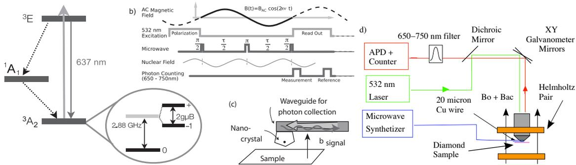
**Figure 1.** Principles of the individual NV electronic spin diamond magnetic sensor. (a) Energy levels for a single NV impurity. (b) Example of the pulse sequence structure of the experimental approach. (c) Scanning tip setup for high-spatial resolution magnetometry. (d) Experimental setup.
