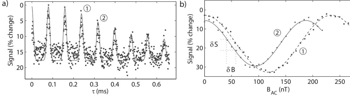
**Figure 2.** Spin-echo-based magnetometry with an individual NV electronic spin in a bulk diamond sample. (a) Example electronic spin-echo measurement (dots) and fitting (solid line, see text). (b) Spin-echo signal as a function of applied AC magnetic field amplitude for two operating frequencies  $\nu_1 = 3.15$  kHz (dashed line) and  $\nu_2 = 4.21$  kHz, corresponding to revivals 1 and 2 in Fig. 2-a.
