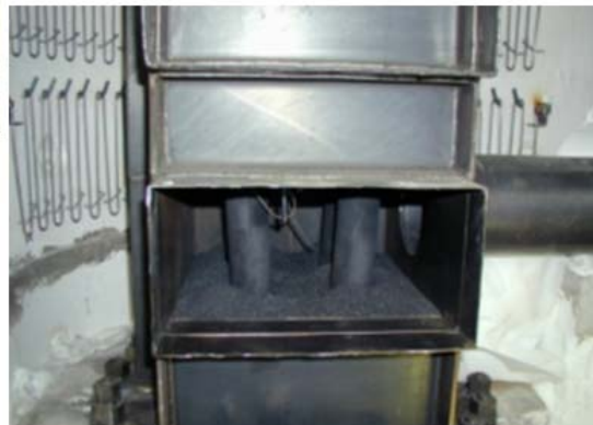
Figure 2-11: Entry chamber, with four graphite columns. On the left, before the experiment, on the right, after the experiment [13]
