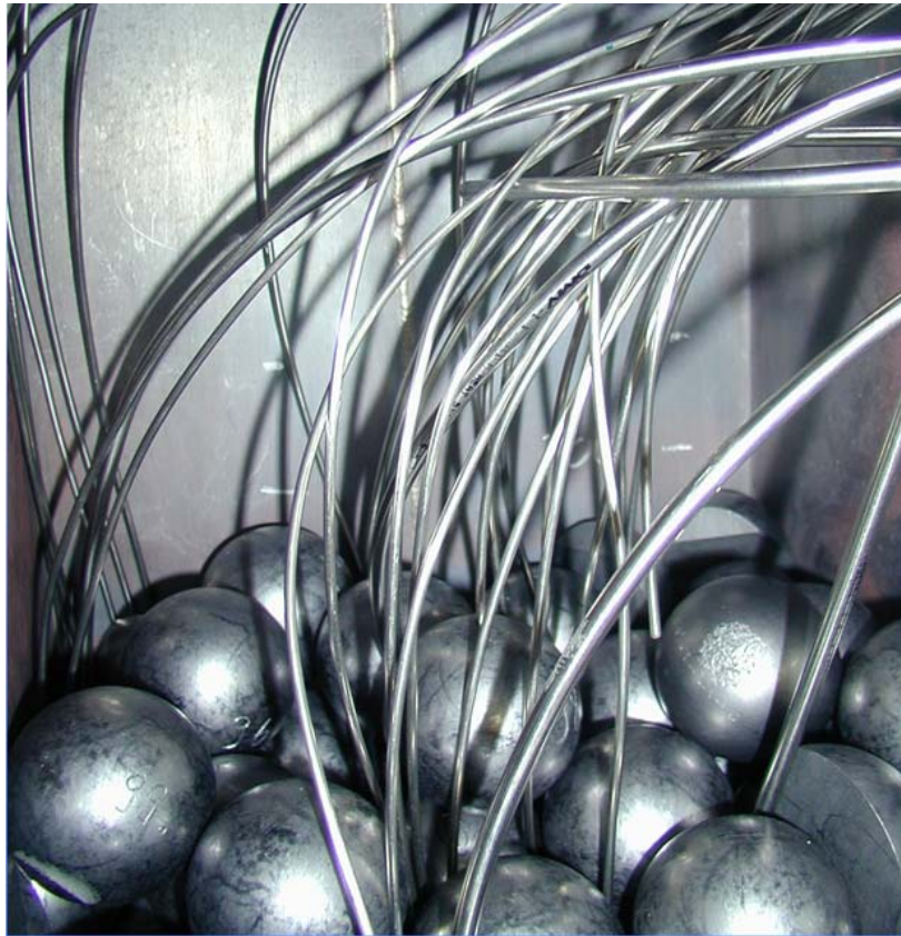
Figure 2-12: 60 mm diameter pebbles. The cables are linked to temperature and species measurement devices located in the lower chimney and pebble bed
