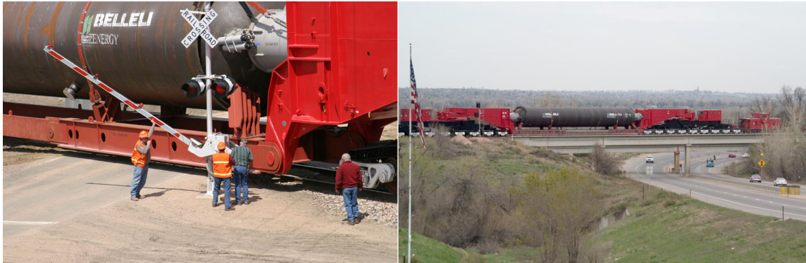
Figure 16: The Schnabel car en route to Commerce City, Colorado from Houston Texas loaded with a 570 metric ton refinery reactor Left: in Trinidad, CO on April 9, 2005 (© Nathan Daniel Holmes 2005) Right: in Larkspur, CO on April 15, 2005 (© Kevin Morgan 2005).
