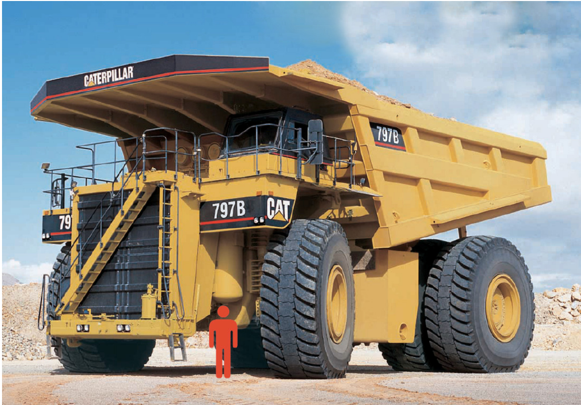
Figure 4: The Caterpillar 797 has a 380 ton capacity and 3370 horsepower. The truck has a 1,800 gallon fuel tank and stands about 25 feet tall by 32 feet wide by 48 feet long. A representative 5'10" tall person is shown for reference.
