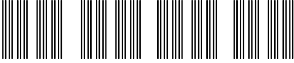
Fig. 6. The data bits are used to sequentially refine a point on a Cantor set. Its natural tree structure allows bits to be encoded sequentially. The Cantor set also has finite gaps between all points corresponding to bit sequences that first differ in a particular bit position. These gaps allow the uniformly reliable extraction of bit values from noisy observations.
