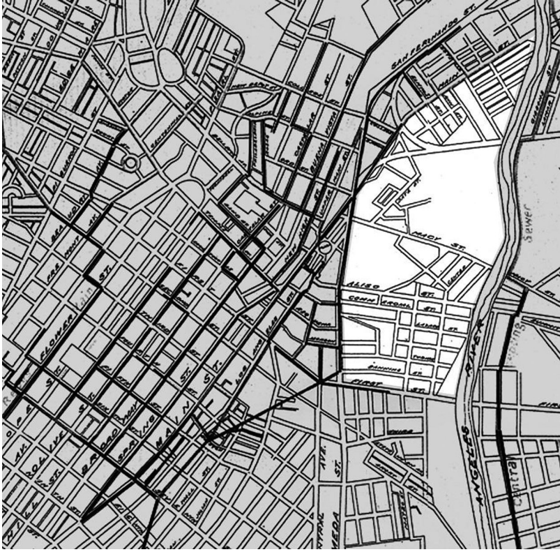
Figure 1. Map “Showing the Varieties and Lengths of Sewers Laid on December 1, 1891,” by J. H. Dockweiler, Los Angeles City Engineer, submitted and bound with City of Los Angeles, Los Angeles Municipal Reports , 1891; the map is bound between pages 53 and 54. The unshaded area indicates the Mexican and Mexican American residential district referred to as Sonora Town; the darker lines represent operating sewers, and the small circle just right of the center indicates the plaza.
