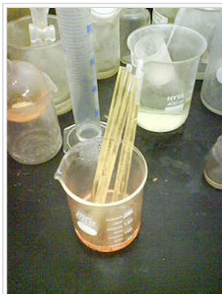
Freshly prepared aqua regia is colorless, but it turns orange within seconds. Here, fresh aqua regia has been added to these NMR tubes to remove all traces of organic material.
