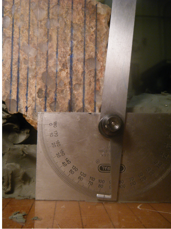
Figure 2-2: Recreating Original Outcrop Dip. EHJH5 was realigned with the original dip and strike measured in the field. A protractor was used to measure this original dip ( 96^\circ ). The blue parallel lines on the rock face represent the up/down direction in true outcrop coordinates.
