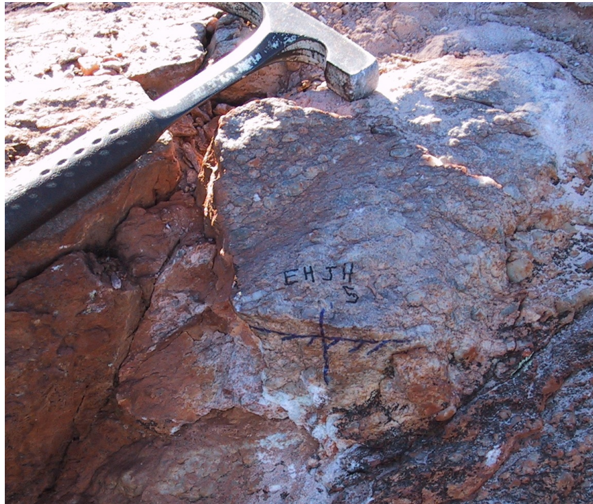
Figure 1-2: EHJH5 before Outcrop Removal. EHJH5 was broken off an outcrop in the Jack Hills Greenstone Belt. A line was drawn on the sample and the right-hand strike and dip was measured relative to this line to be 92^\circ and 96^\circ respectively.
