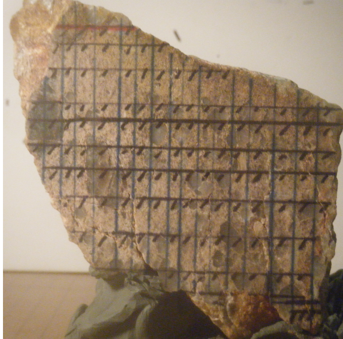
Figure 2-3: New Grid System on Flat Side. Lines were drawn on the flat side of EHJH5 after the side's strike and dip were measured. Acrylic was glued on the side shown to help prevent crumbling when the sample was cut.
