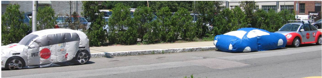
Figure 2: Experimental set-up for Active Park Assist™ (APA) assessment with balloon cars at either end of designated parking location.
