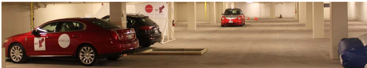
Figure 3: Experimental set-up in a parking garage for the Cross Traffic Alert (CTA) evaluation with a mid-sized car directly adjacent to Lincoln MKS test vehicle and then a white screen with the dimensions of a panel truck further obscuring the research subject's view. The confederate vehicle used to set-off the CTA warning can be seen in the background along with the rear of a balloon car at the right.
