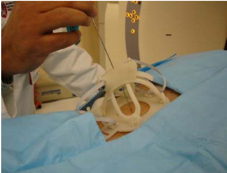
Mock-up of the Robopsy device on a patient.
