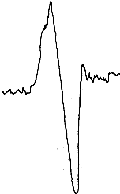
Fig. 10. EPR spectrum from roughly 10^{13} free radicals in the cavity resulting from \gamma -irradiation.
