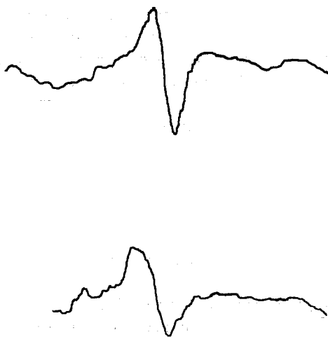
Fig. 15. Spectra in nylon 66 resulting from \gamma -irradiation at liquid nitrogen temperatures and then subsequently annealed at room temperature: (upper curve) annealed 1 min; (lower curve) annealed 6 min.
