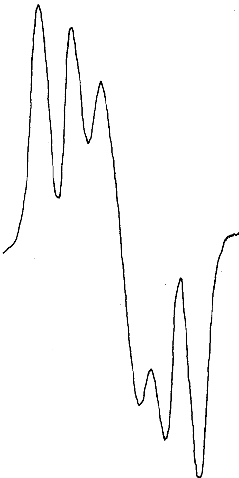
Fig. 2. Typical spectrum obtained during tensile loading to fracture of nylon 6 fibers.
