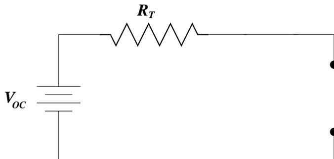
If you know what the big mess inside the “black box” is made out of, then you can figure out  $V_{OC}$  and  $R_T$  as we did for the example above.
