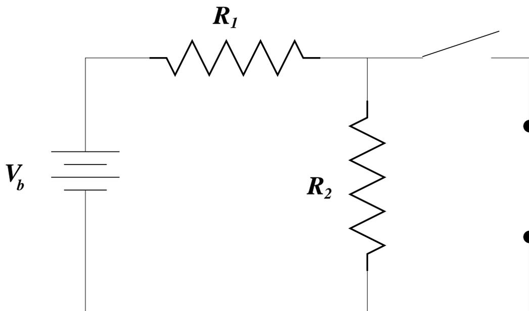
If we short circuit these terminals with a wire, a current  $I_{SC}$  — the “short circuit” current — will flow. On the other hand, if we leave it open, there will be a potential difference — the “open circuit” voltage,  $V_{OC}$  — between the terminals (equivalent to the potential drop over the resistor  $R_2$ ).
