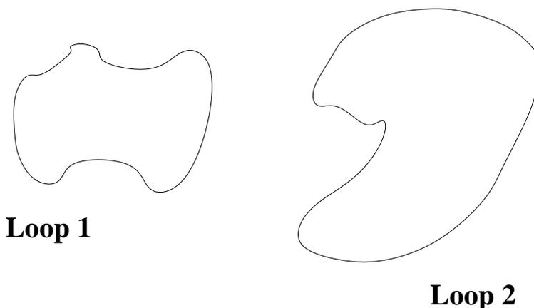
Suppose that a current  $I$  runs through loop 1. What is the flux of magnetic field through loop 2 due to the current in loop 1? By definition, this flux will be
