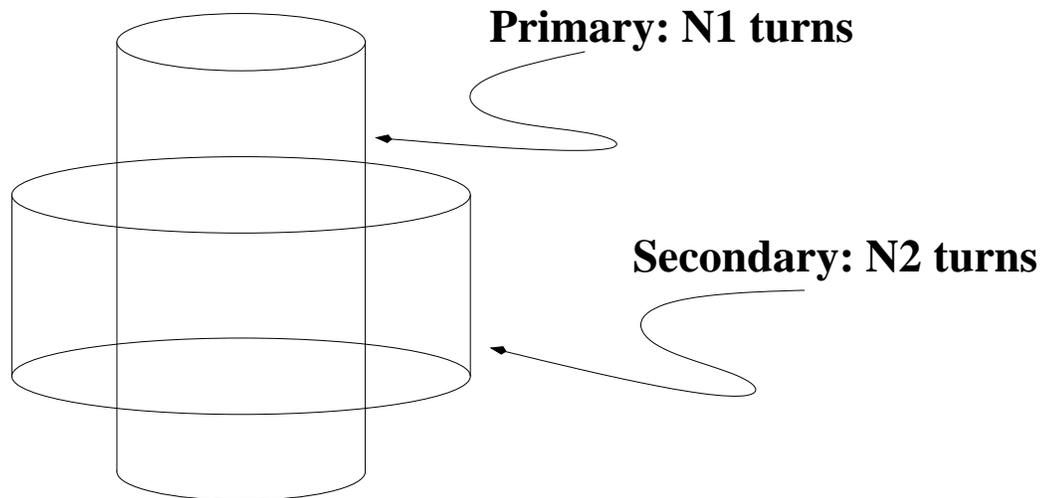
The idea is that we drive a time varying current through the primary, making a time varying magnetic flux:
