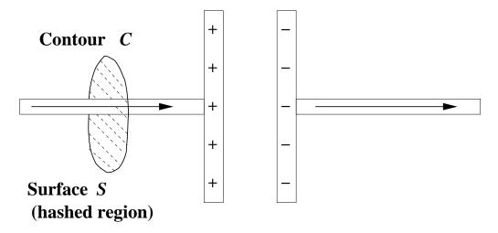
The current  $I_{\rm encl}$  is then just the current I flowing into the capacitor. Nice, simple, logical.
