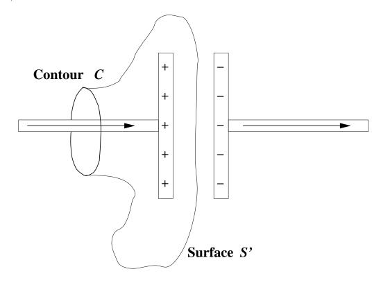
The amount of current flowing through this surface is ZERO: no charge flows between the plates! However, there is a flux of *displacement current* between the plates. When we turn our "generalized Ampere's law" into an integral form, we get
