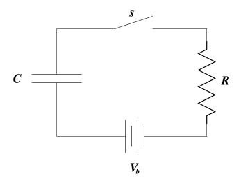
As the capacitor charges up, a displacement current flows between the plates. As a consequence, a *magnetic* field is induced between the plates, in addition to the electric field that is building up. We'll now calculate this magnetic field.
