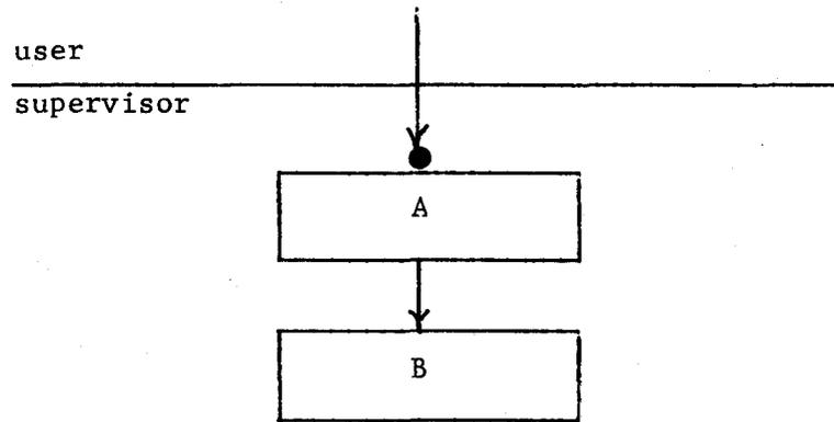
A and B are procedure modules in the supervisor. Imagine that a single invocation of A (by a user procedure) can result in a flurry of calls from A to B. Then there is a clear performance cost in moving the user/supervisor boundary to between A and B, even if only B need be part of the protected, common supervisor.
