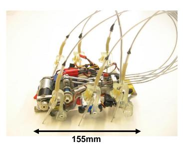
Fig. 1. iSprawl: a fully autonomous hexapedal robot driven by an electric motor and flexible push-pull cables.
