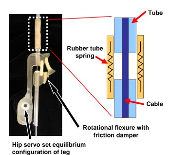
Fig. 4. Schematic of the leg compression spring design utilizing a tension spring in the flexible tubing around the push-pull cable. Also shown are the frictional dampers (on front and middle legs).
