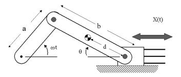
Fig. 11. Schematic of Crank and Slider
