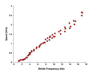
Fig. 7. Running speed of iSprawl vs. stride frequency
