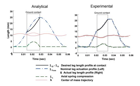
Fig. 6. The theoretical and experimental leg extension profiles for iSprawl running at  $2.3 \ m/s$ . Also shown are the path of the COM and the extension of the axial spring for each case. The dashed line in the analytical plot shows COM trajectory that would occur without any spring compression. Curves for the measured leg extension and COM trajectory represent averages of three successive strides shown in gray dots.
