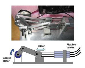
Fig. 2. Power transmission system for *iSprawl*. A double crank-slider is used to store and convert the rotational energy from the motor to linear oscillations.
