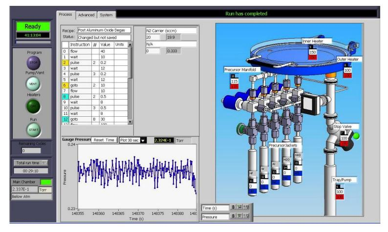
The process chamber is kept under vacuum and must be vented to load your sample.
