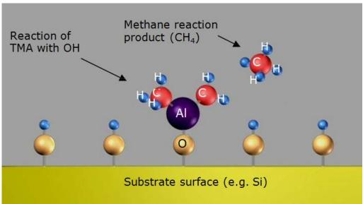
Step 2: Removal of the unreacted precursor and reaction products. Unreacted precursor and the methane (CH<sub>4</sub>) liberated from the reaction are removed by simple evacuation of the sample chamber or by flowing inert gas over the surface.
