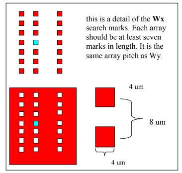
The center mark in the array defines the position of the mark in the process program.
