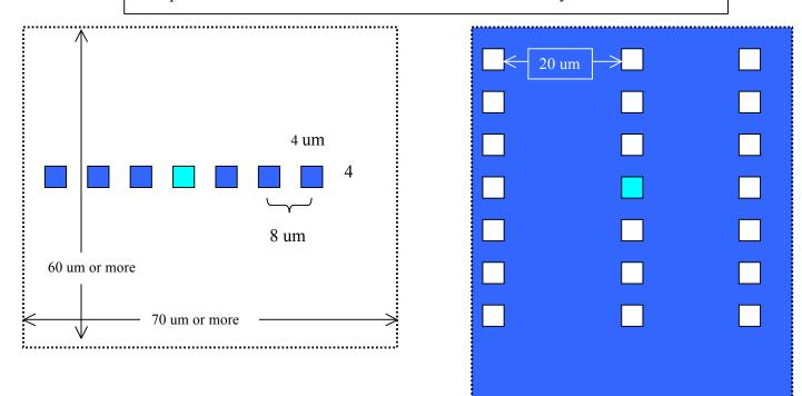
Arrays should be a minimum of seven marks long. The center mark defines the array position in the process program. Either array tone's center mark may serve as LSA target.
