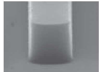
An AZ® MiR 701 resist pattern after a baking step at 130°C. Due to the high softening point of approx. 135°C, no rounding becomes visible.
