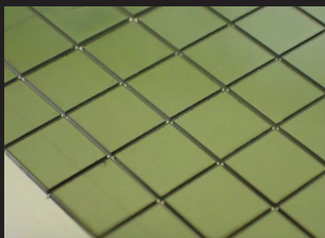
Silicon Carbide (SiC) device singulation by laser. 100um-t, 3mmX3mm
