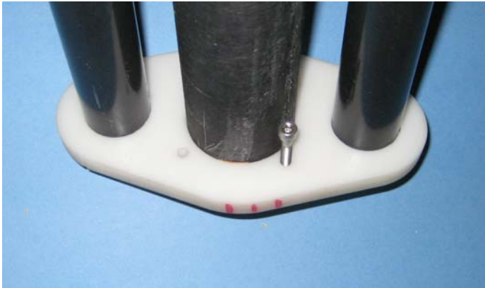
Figure 2. Model riser clamp with carbon fiber main pipe and water injection lines. The screw is for setting the angle of attack.
