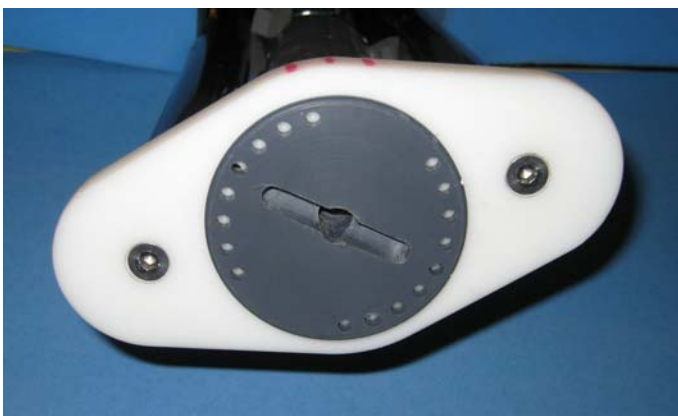
Figure 3. Gray PVC end plug with central mounting hole and anti-rotation slot. The circle of small holes was used to set the angle of attack of the model riser relative to the incoming flow.
