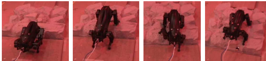
Fig. 8. LittleDog using a dynamic lunge to get onto elevated rough terrain.
