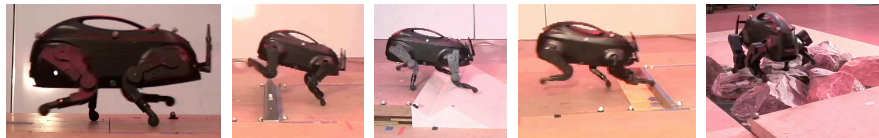
Fig. 5. LittleDog traversing various terrain dynamically.
