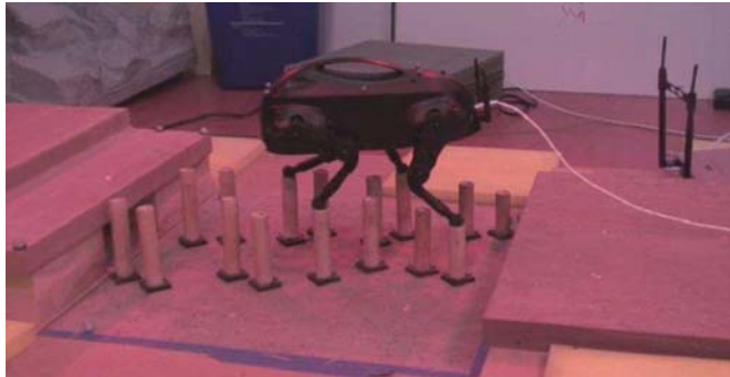
Figure 1: LittleDog robot, which can navigate intermittent terrains which require careful foot placements.
