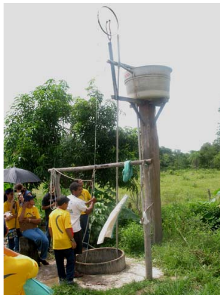
Figure 18. GSR students demonstrate the water extraction device they built in the settlements.
