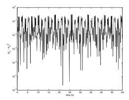
When varying these sets of initial conditions slightly, we find very little difference in the resulting motion, showing a stable region of the dual pendulum's behavior. The error terms are small, and do not grow with time.
