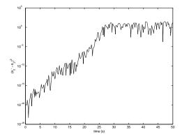
The squared difference between  $\theta_2$  in two runs with initial conditions varying by an angstrom is shown above. The log of the error increases roughly linearly with time, until reaching its maximum error of
