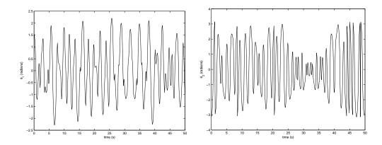
The two graphs above show the two pendulum angles over the 50 second experiment.
