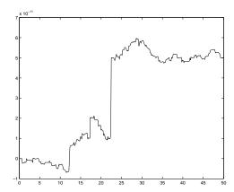
The above graph shows the total energy of the system as a function of time. It stays below  $10^-10$  J, which is a reasonable conservation. The error is induced from errors accrued in numerical integration.
