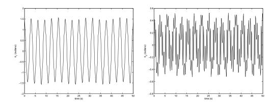
With differing initial conditions, the dual-pendulum system acts almost periodically. The first pendulum has roughly sinusoidal displacement, while the lower pendulum has smaller periodic oscillations.
