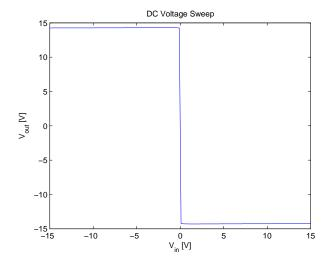
The DC sweep shows that the output swing is  $\pm 14.3$  V, and that the output current is  $\pm 14.3$  mA. By decreasing the load resistor to 10  $\Omega$ , we find that the maximum output current is  $\pm 250$  mA.
