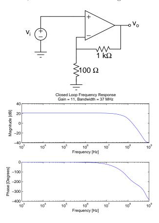
The frequency response of the closed loop system shows that we achieve the expected gain of 11 from the amplifier, with a bandwidth of 37 MHz.
