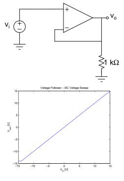
By using a voltage buffer, we can show that the amplifier can handle common mode inputs sweeping almost from rail to rail, with a common mode range of  $\pm 14.8 \text{ V}$ .
