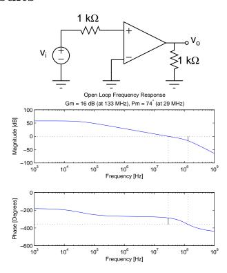
In the graph above, we see the results of simulating the amplifier running open loop. The low frequency gain 58 dB implies an open-loop transimpedance of 800 k $\Omega$ . To achieve the required phase margin, a 3 pF capacitor is connected to the high impedance node in the amplifier, raising the phase margin to 74°.
