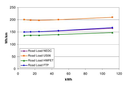
Energy Consumption vs. battery capacity
