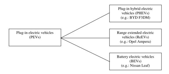
Fig. 2.1 Plug-in Electric Vehicle classification
